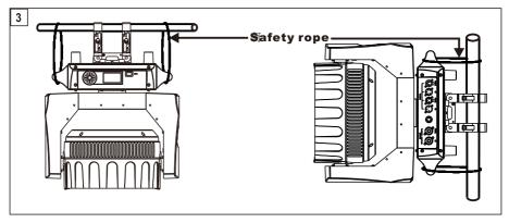
Installing the projector- Fig. 3
